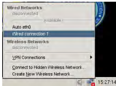
Figure 19 — Initiating a Static IP Connection
